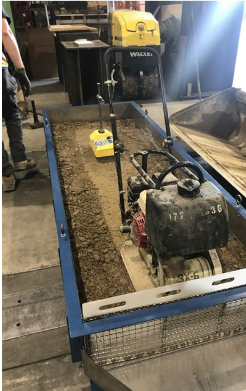
Figure 4.2 Compaction of gravel aggregate into roadbed test frame. Vibratory plate tamper used to achieve desired % compaction. Nuclear meter used by CMT Labs (State College, PA) to confirm % compaction in relation to number of tamper passes.
