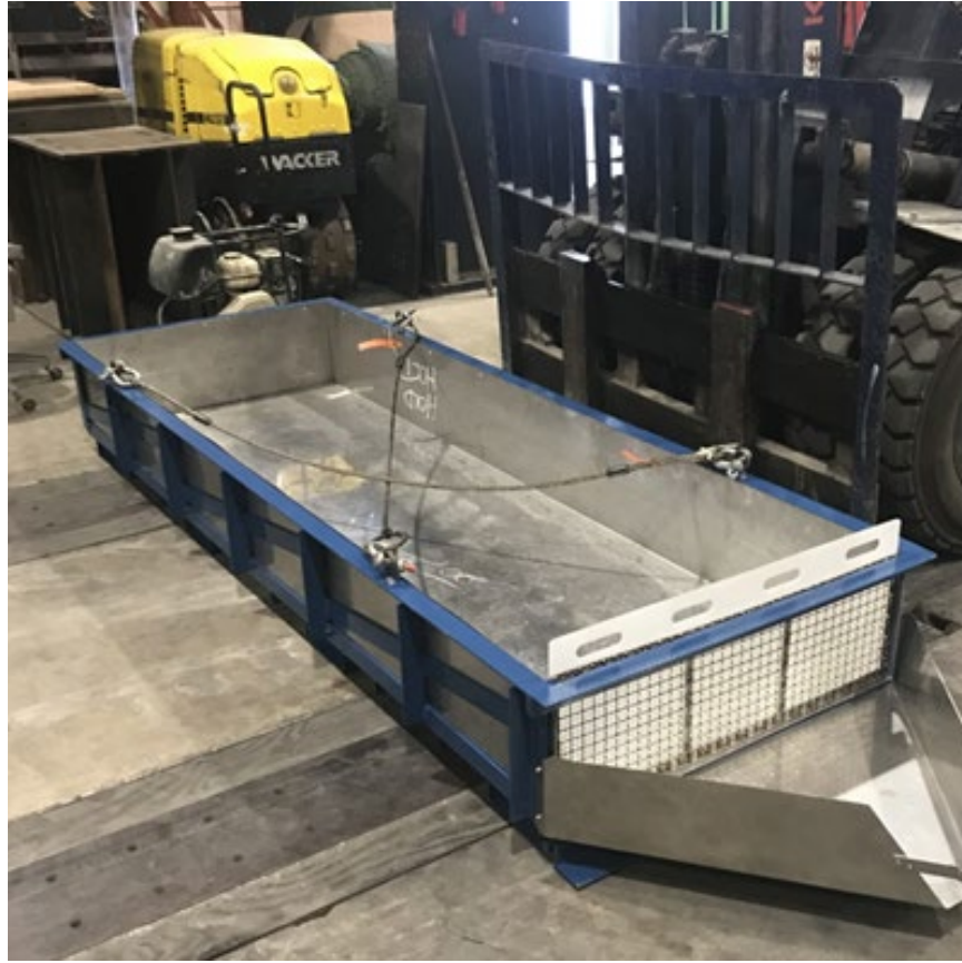
Figure 4.1 Roadbed test frame. 3-foot wide, 9-foot long, stainless-steel lined. Crossed cables used to assist with lifting frame onto steel I-beams. Plastic endpiece removed after roadbed was compacted into test frame. Stainless-steel discharge chute conveyed runoff into flow-through sample bucket.
