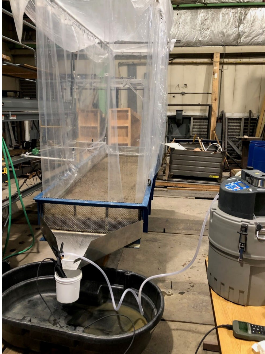
Figure 4.4 Sampling equipment positioned at downstream end of roadbed test frame. 2-gallon plastic bucket was hung onto end of discharge chute. Overflow from bucket was captured in large black plastic tank on floor. Hannah multimeter and ISCO sampling tube were fastened into sampling bucket. Rainfall nozzles positioned inside shower curtain enclosure. Rainfall pumping equipment mounted on scaffold next to test frame.
