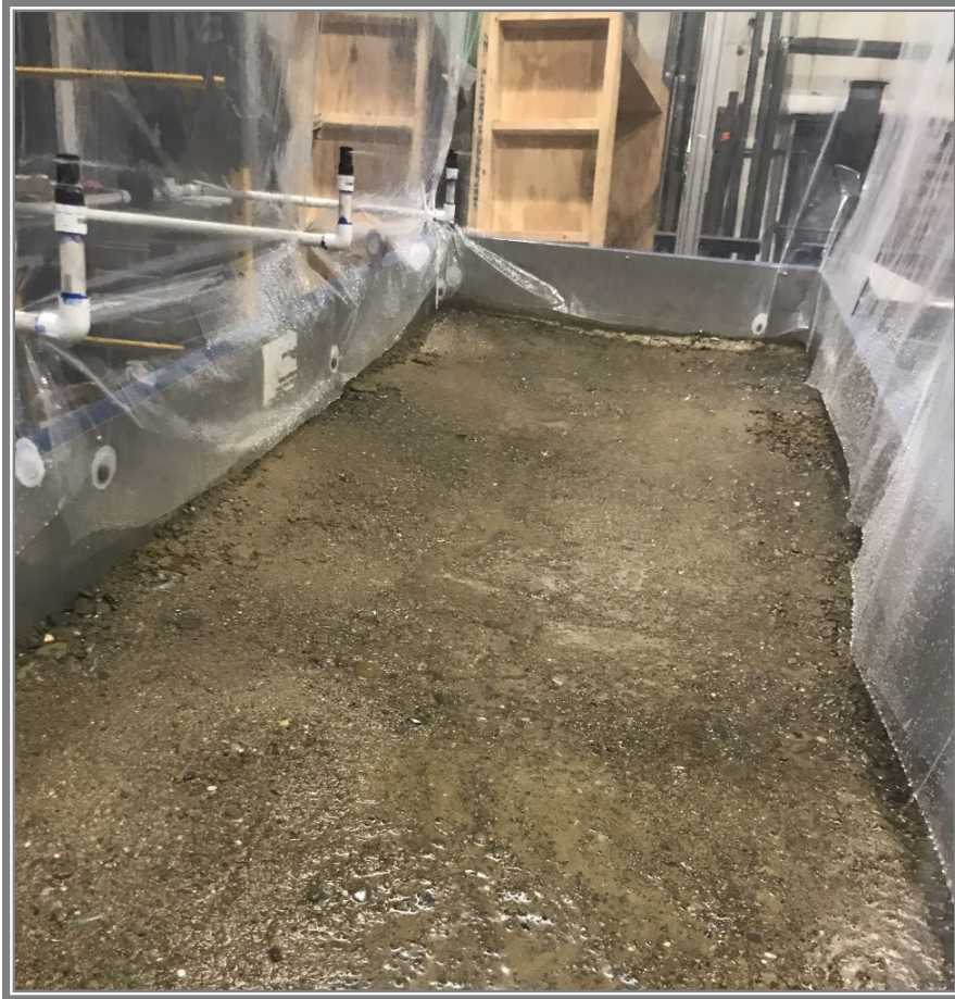
Figure 4.5 View of rainfall nozzles positioned inside of shower curtain enclosure. Each nozzle delivered synthetic rainwater evenly across a 3-foot by 3-foot square section of the roadbed. Shower curtains contained any over overspray and retained humidity.
